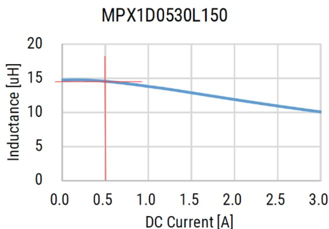
Figure 3 – Buck Inductor Rating
