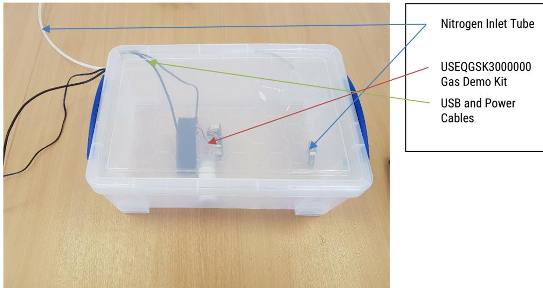
Figure 1 – USEQGSK3000000 Gas Demo Kit in Nitrogen Filled Container
